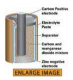
Regular disposable AA and AAA batteries are considered Primary Cells, and are most widely recognized as conventional "alkaline" batteries. There are two electrodes inside each cell; one is made of Zinc, known as the anode (the negative terminal) and the other is made of Manganese Dioxide, known as the cathode (the positive terminal). The electrodes are surrounded by an alkaline electrolyte, the chemical from which alkaline batteries get their name.
